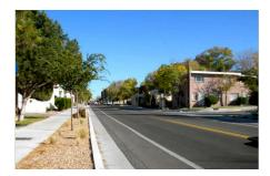
A Complete Street: this street includes a shaded, landscape buffered sidewalk, providing a flat, protected place to walk. The bike lane allows for safe bicycle access while the single lane in each direction allows the prudent driver to set the speed.
