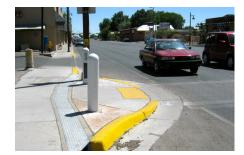
Bulb out + textured crosswalk: bulb outs help to visually and physically narrow the street. This creates a) a shorter crossing for pedestrians and b) reduced vehicle speeds. The textured crosswalk defines pedestrian space, commanding more respect from automobile drivers. Location: Bernalillio, NM.
